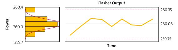
Using these results, our solar panels are categorized according to performance during a process we call "plus-sorting." Only those panels that demonstrate a nominal power performance or higher move forward, making this process synonymous with the highest level of efficiency.
