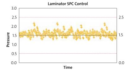
The quality of EVA and the level of curing in the lamination process is paramount in the long-term durability of the module and protecting the electrical circuit made up by the cells. By monitoring our lamination process with SPC, we can ensure that the lamination of the EVA is on target for each module and that they will stand the test of time.
