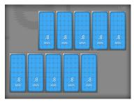
This section of the screen displays an aerial view of the roof, showing how the solar modules are physically configured. The homeowner can view energy production information for each module on a current, daily, monthly and lifetime basis.
