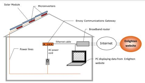
The Enphase Envoy Communications Gateway is an integral component of the SunSource® Home Energy System. It operates between the microinverters on the Solar Modules and the Enphase Enlighten™ Performance Monitoring website and analysis system. The Envoy functions as a gateway and monitors the microinverters that are connected to the modules.
