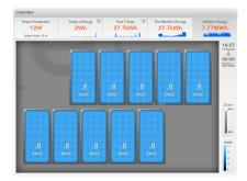
The overview pane displays current system status, current energy production, the energy produced for the day, the month and the lifetime of the SunSource system.
