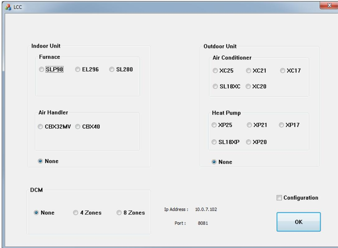
2. At the bottom of this screen to the left of the *OK* button, the *IP Address* and *Port* settings are displayed. Make a note of these values. This address will change each time your computer connects to a different IP address and this step will need to be repeated.
