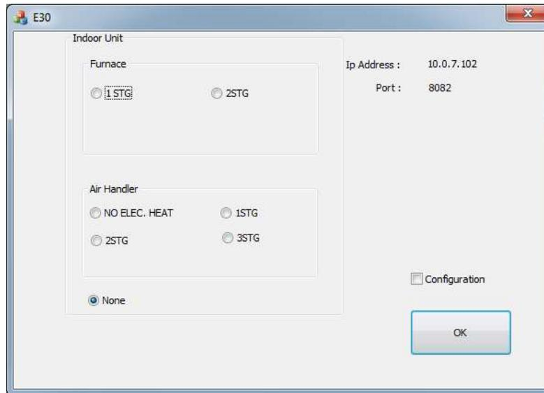
2. At the top right corner of this screen the IP Address and Port settings are displayed.
